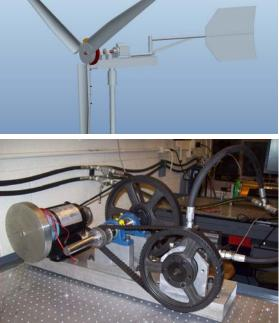
Figure 2 (top). CAD model of wind turbine nacelle. Figure 3 (bottom). Electric generator driven by the hydraulic motor through a synchronous belt drive.
