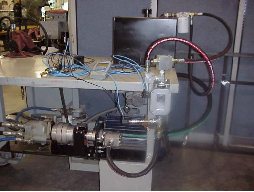
Figure 1, Pump efficiency test bench.
