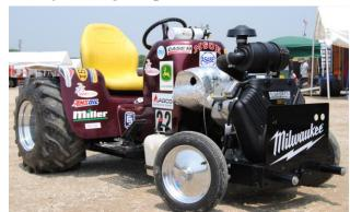
**Figure 3:** Picture of 2011 EHPP model at 2011 IQS competition in Peoria, IL. One can notice the unsafe location of the fuel tank behind the right front wheel as well as the single-piece fiberglass body.
