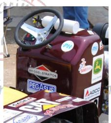
**Figure 4:** Picture showing poor control labeling and layout along with lack of instrumentation on 2011 EHPP.
