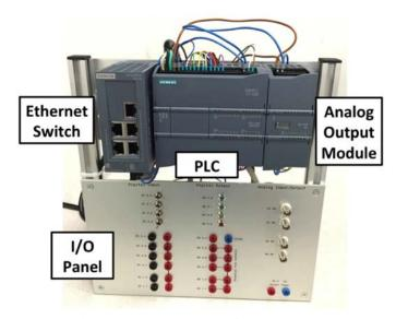
Figure 1. ME6404 PLC Test Panel
