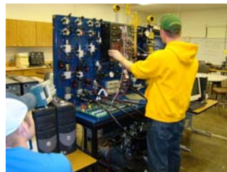
Picture 2: An Iowa State Agricultural and Biosystems Engineering student uses a PLUS+1 development board to link the electronic control module to an electro-hydraulic trainer. The PLUS+1 controller received cylinder set point commands from a CAN Bus interface, operated solenoid valves to manipulate the position of a hydraulic cylinder, and monitored the cylinder position with an in-cylinder position sensor.
